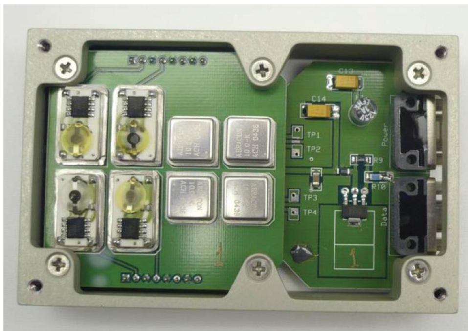
Figure 4. Photograph of quartz crystal microbalance flight package that was exposed to the low-Earth-orbital environment on MISSE-6 (PEC-B, ram direction). Four quartz crystals, each with a diameter of 8 mm, may be seen. During the exposure, an aperture of \sim 6 mm diameter limited the exposed region to the central portion of each disc. Clockwise from upper left: 0 wt % \text{Si}_8\text{O}_{12} SC POSS polyimide, 7 wt % \text{Si}_8\text{O}_{12} SC POSS polyimide, 20 wt % \text{Si}_8\text{O}_{12} SC POSS polyimide, and fluoropolymer (part of an unrelated experiment). The polyimide films were roughly 2 \mu\text{m} thick. Close inspection indicates that the 0 wt % POSS polyimide was eroded away completely in the exposed region, while the POSS-containing films were not eroded away.
